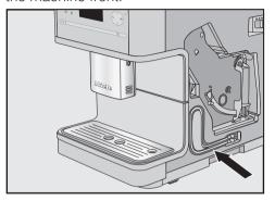
■ Connect the milk pipe to the aperture in the main dispenser.
